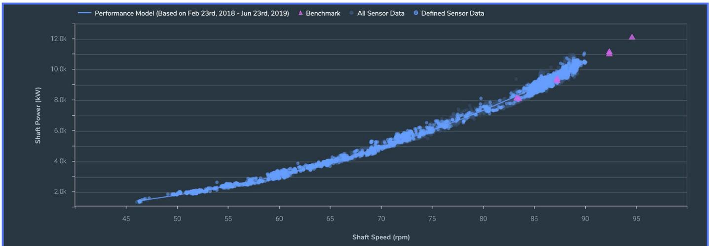
Nautilus Platform implements advanced machine learning techniques that quantify the relationship between shaft speed and shaft power—based on each vessel's historical performance. By stripping and reapplying a ship's range of potential weather and draft
